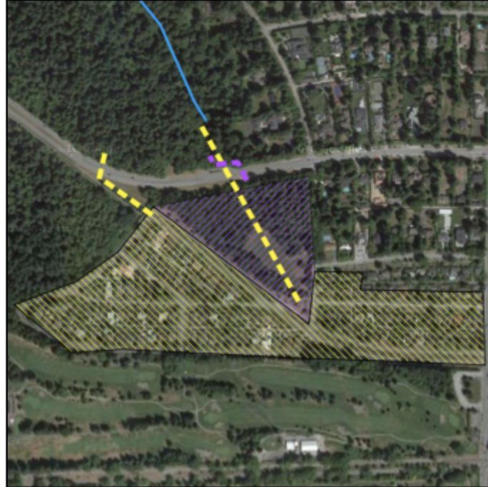
Figure 9: Three culverts drain into the watershed of Spanish Bank Creek. These culverts are indicated by the dashed lines. The polygons indicate the approximate areas that the culverts drain and are paired to the culverts according to colour. The yellow polygon is 12.8 ha, and the purple polygon is 4.7 ha (QGIS Development Team, 2009).
