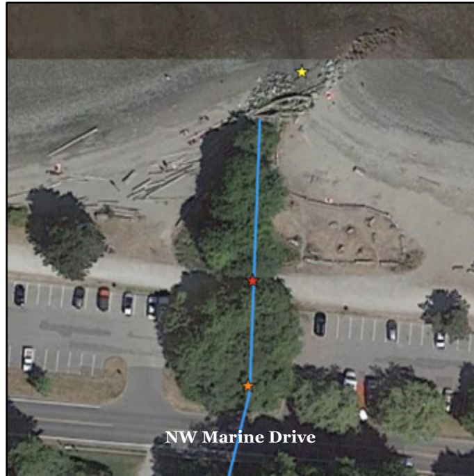
Figure 26: Locations of sediment removal for the lower reaches of Spanish Bank Creek. The first priority is the culvert under the footbridge (red star). The second priority is the pre-cast concrete headwall at the north end of the wood stave culvert (orange star), and the last priority is the mouth of Spanish Bank Creek to re-grade the lower reaches of Spanish Bank Creek (yellow star; QGIS Development Team, 2009).
