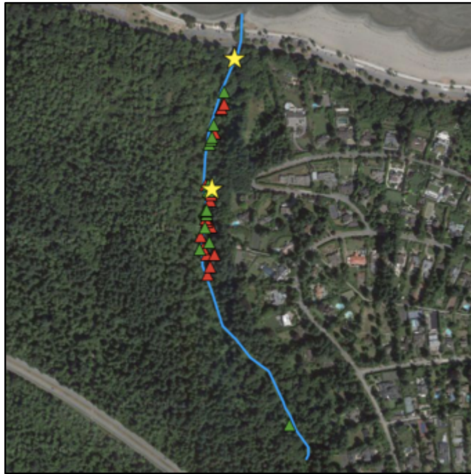
Figure 12: A map of inputs into Spanish Bank Creek. Green triangles represent the 14 runoff inputs from bank left, red triangles represent the 18 runoff inputs from bank right. Yellow stars represent the two drainage pipe inputs into Spanish Bank Creek. Field work was conducted on 4 November 2016 (QGIS Development Team, 2009).
