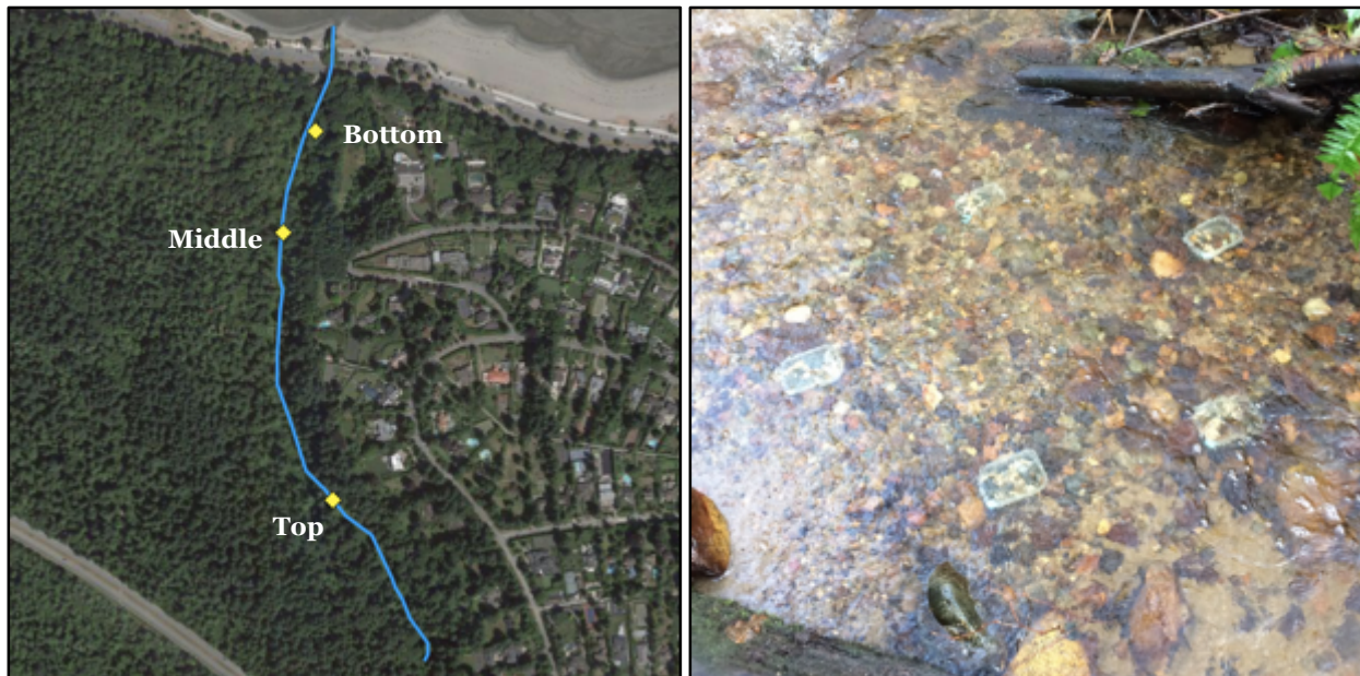
Figure 7: Fifteen sediment accumulators were installed in Spanish Bank Creek. The sediment accumulators were installed in Spanish Bank Creek at locations denoted as top, middle, and bottom (left; QGIS Development Team, 2009). Five accumulators were installed at each of the locations, for a total of 15 accumulators (right; Reynolds, 2016).
