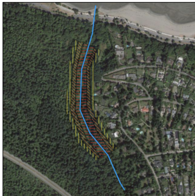
Figure 25: Location within Spanish Bank Creek where the soil bioengineering techniques will be installed. Brush layers will be installed upslope (yellow polygon), live gully breaks will be installed midslope (orange polygon), and live stakes will be installed downslope (red polygon) along the edge of Spanish Bank Creek (QGIS Development Team, 2009).
